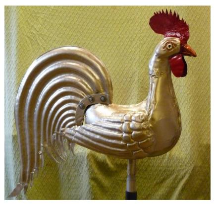
The damage was considerable and deciding how to repair it was not easy. It is made from copper, which hardens when it is bent so is liable to crack when bent back. Before attempting to bend it back it is best to anneal the copper, but this entails heating it to 700 degrees centigrade and letting it cool, at which temperature all the solder and lead would have melted and run away.
